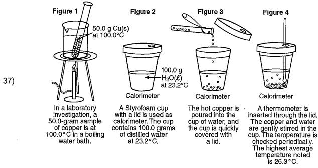
In terms of energy flow, explain why the temperature of the water in the calorimeter used in the investigation shown increases.
