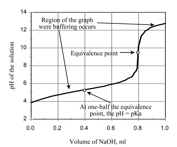
**Equivalence Point** - At the equivalence point, the number of moles of aqueous hydrogen ion, H<sup>+</sup>(aq), which have been neutralized by exactly the same number of moles of aqueous hydroxide ion, OH<sup>-</sup>.
