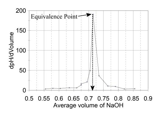
To prepare the first derivative graph, calculate the slope () pH/) Volume) and average volume of titrant within  $\pm 0.15$  ml of the predicted equivalence point. Note the sample calculations in the table below.
