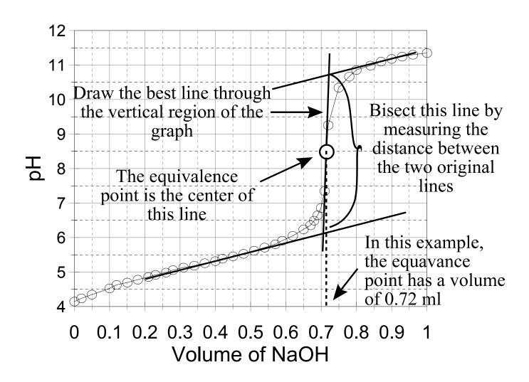
Drop a line perpendicular to the x-axis at this point to determine the volume of titrant added to reach the equivalence point. Once this value is known, the concentration of a monoprotic acid may be determined from the relationship:
