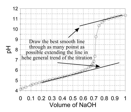
Step 2. Draw a line through the portion of the graph with the greatest slope. Measure the length of this line between the two lines drawn in Step #1, and find its center. The center of this line is approximately the equivalence point.
