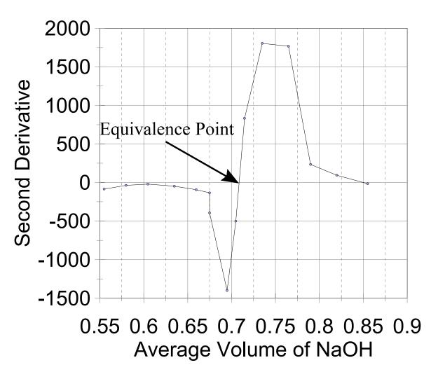
In the second derivative graph, the change in the slope from the first derivative data table () pH/) volume) is plotted against the change in the average volume. The equivalence point occurs where the change in the slope is zero. Observe the adjacent second derivative plot.
